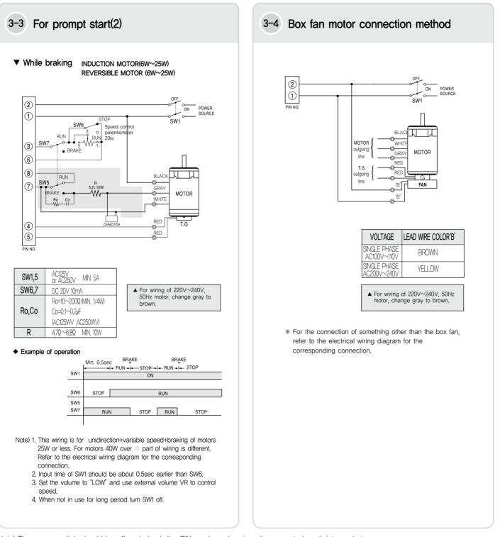
Note) The power switch should be off and check the PIN number when inserting a control pack into socket groove. (There is a possibility to be burned.)
