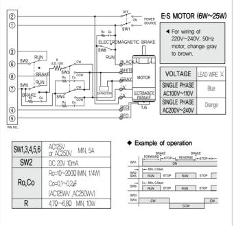
When electric brake of controller is used at the same time
